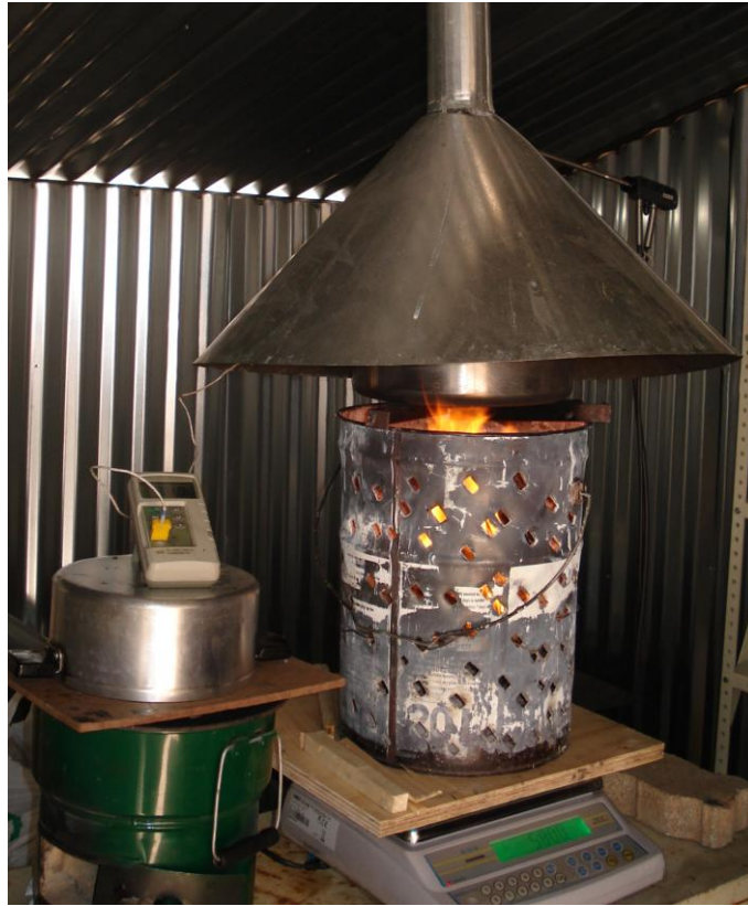
Testing an imbaula stove at the SeTAR Centre
