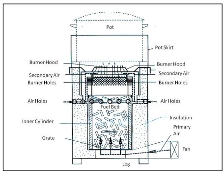
insulation to prevent escape of heat through the surface of the stove body. The primary air enters from the bottom end of the reactor with the use of a 0.15-Amp, 12-V DC fan. The secondary air, on the other hand, enters the reactor through the holes in the middle of the stove body and is mixed with the gas generated at the small holes located at the upper portion of the burner. A skirt is sometimes provided for the stove to increase heat transfer efficiency to the cooking pot.
