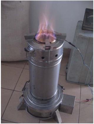
rectangular holder that support the pot in place during cooking, a burner plate that distributes the gas for even heating, air holes for the entry of the secondary air needed for the combustion of gas, and a handle for ease of removal of the burner especially when reloading fuel. The reactor assembly is where rice husk is gasified by introducing limited amount of air, just enough to
