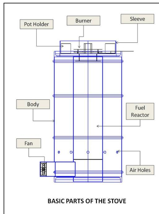
and the burner; (c) the fan, which uses DC 12 volt, 2 watt supplies the required air to gasify rice husks. The flame coming out of the burner is bluish in color, which indicates a very clean gas. It has low black carbon emission of about  $50 \text{ ug/m}^3$  and below. The  $\text{CO}_2$  emission is about  $0.6 \text{ kg CO}_2$  per kg rice husks.
