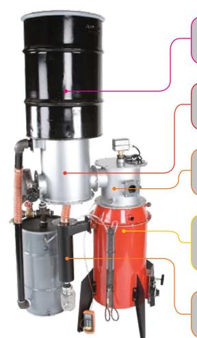
**Hopper:** Air tight hopper holds enough biomass for 4-6 hours of runtime.
