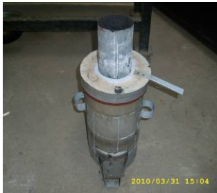
Figure 2.1: The “Champion-2008” TLUD gasifier stove
