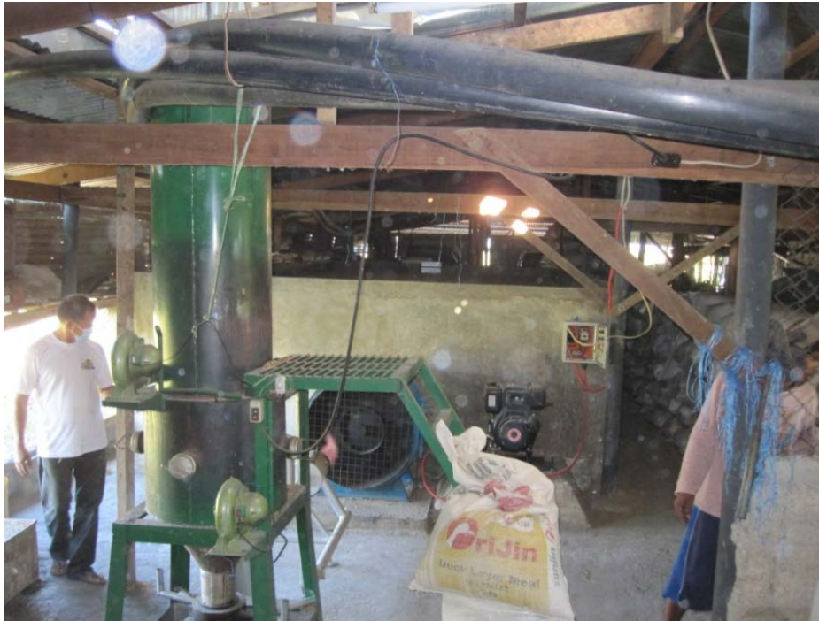
Figure 3. The CFRHG Model-40D Used for Drying Paddy Seeds in Nueva Ecija, Philippines.
