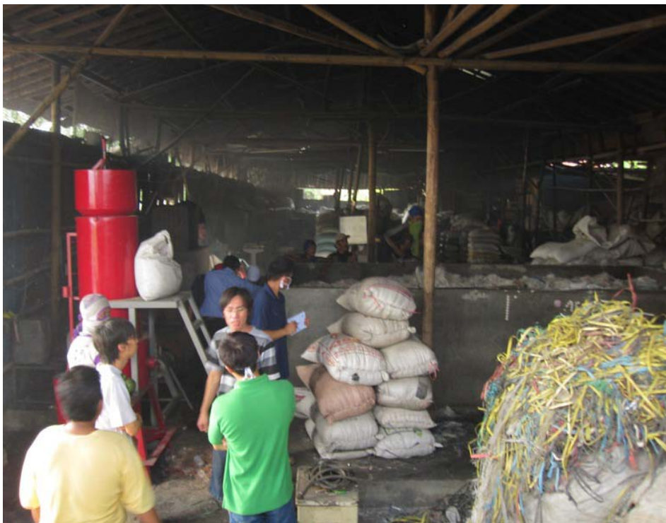
Figure 4. The CFRHG Model-45D Used for Drying Shredded Plastics in Tangerang, West Java, Indonesia.
