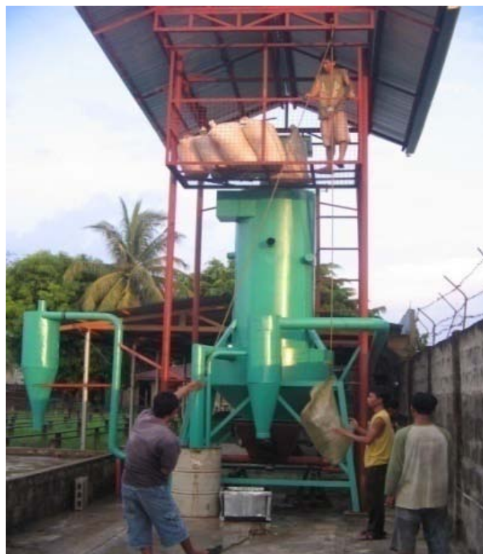
Figure 6. The CFRHG Model-80D Used for Drying Food Products in Tarlac City, Philippines
