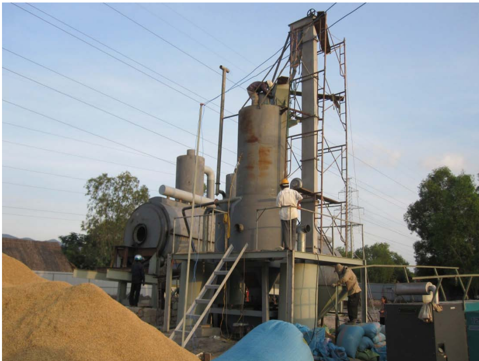
Figure 8. The CFRHG Model-120D Used for Torrefying Rice Husks in Vung Tau Province, Vietnam.
