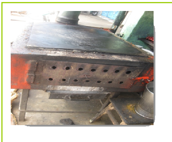
The Kriya Tava stove is a multipurpose stove and can be used to prepare dosas, chapattis, parothas, omelettes etc (terminology for local Indian cuisine). It comes with folding legs which help in moving the stove. It has well designed fins on the lower surface of the tava (flat plates) which ensures a uniform tava temperature.
