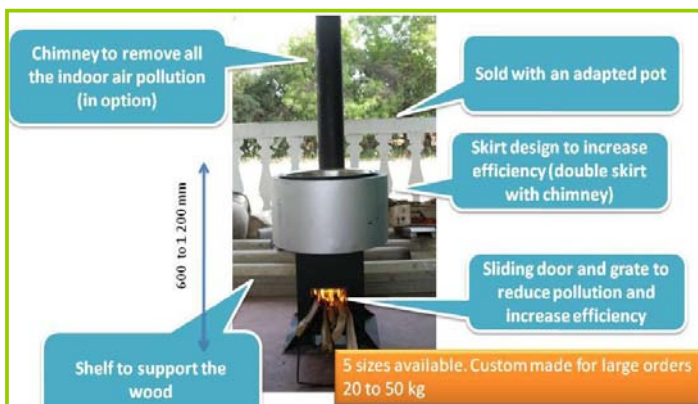
Annotated MOBY Stove designed by Prakti Design and manufactured by Skill Mech (Chennai)
