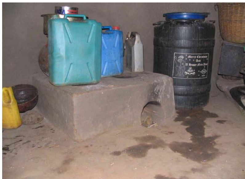
Figure 11: Lorena stove being used for storage
