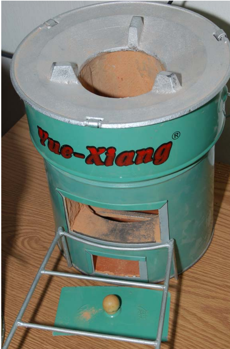
Figure 8: Chinese rocket stove. For this test, a gas burner similar to that shown in Fig. 1 was placed in the area where the wood would normally burn.
