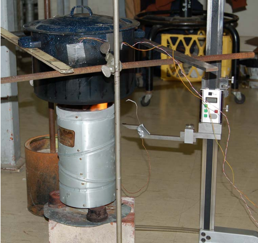
Figure 5: Simulated rocket stove. The burner inside the duct (riser) is the same burner shown in Fig. 1.
