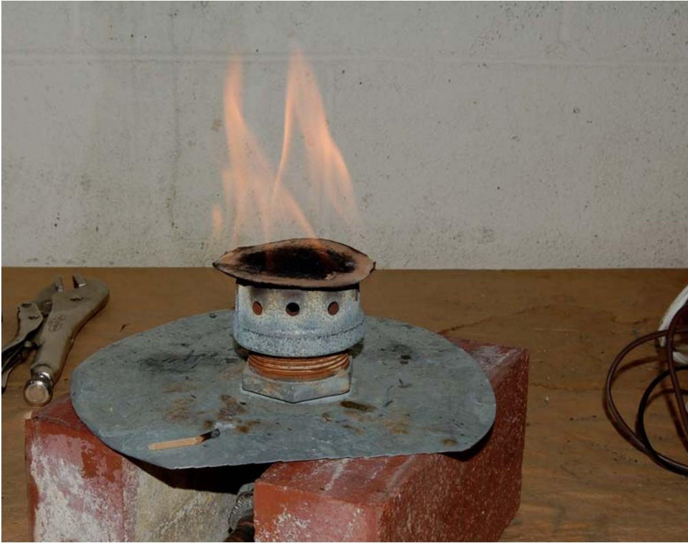
Figure 1: The basic burner being used as a simulated open fire.
