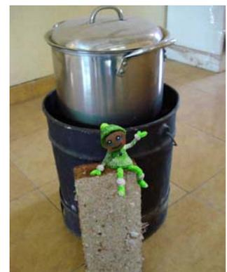
The stove will be custom designed for The Gambia's conditions taking into account the maximum size of a standard domestic cooking pot and dietary requirements. It only comprises of 4 simple parts, its use is easy to learn and safe and it can be manufactured with tooling available on an industrial and local level from new or used steel and parts.
