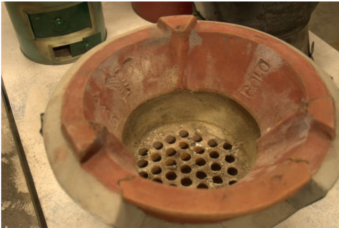
Photo 16: Fuel bed and pot supports of Lao Bucket.
