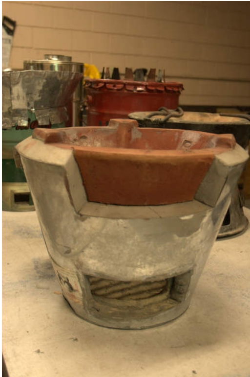
Photo 14: Air intake of Lao Bucket.
