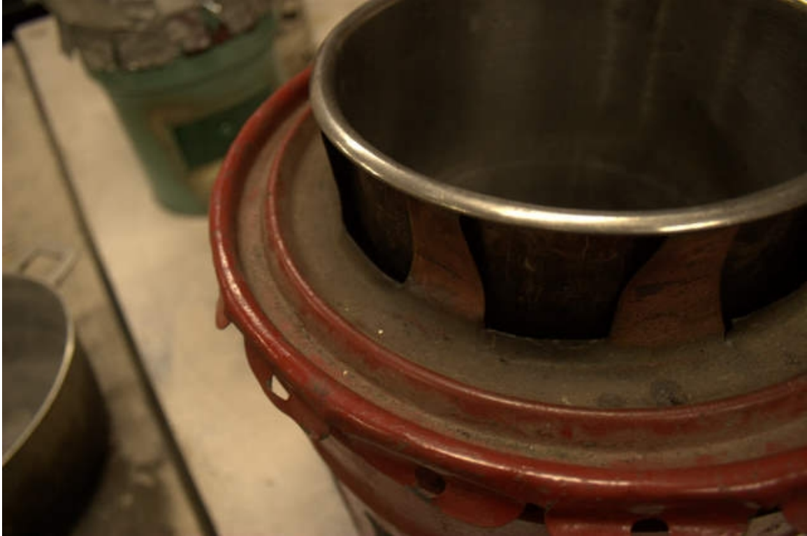
Photo 9: Close fitting skirt of the Henson.
