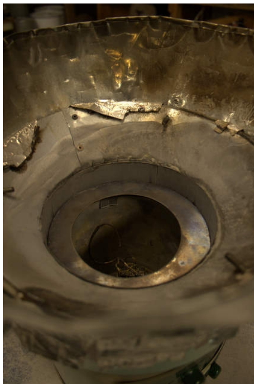
Photo 5: Secondary air control plate and pig tail of Yue Shwing.
