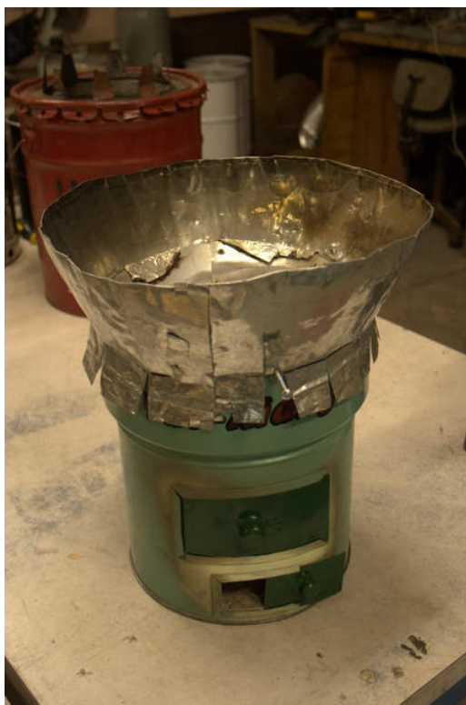
Photo 6: Yue Shwing with partially open door and pot specific skirt.
