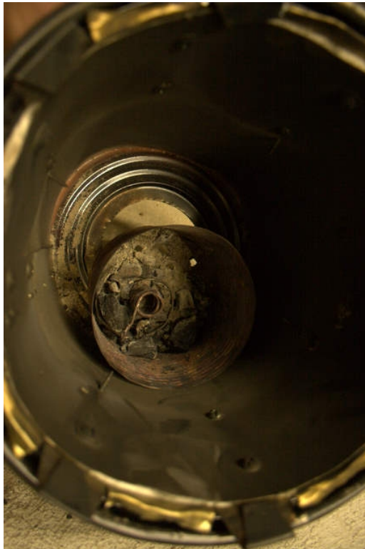
Photo 18: Fuel canister with pig tail offset to show air intake of 5L Henson.
