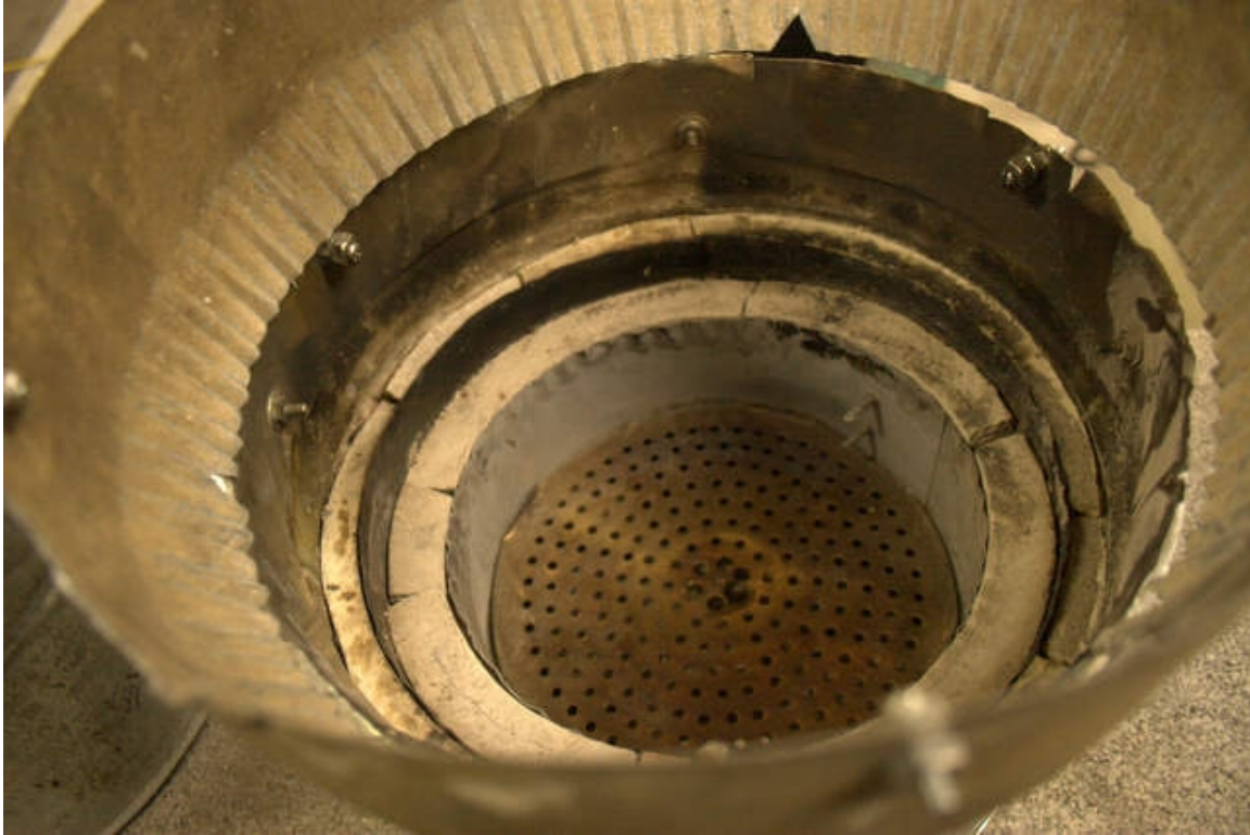
Photo 12: Perforated reflector plate of Mamamusa with rock wool wall insulation.
