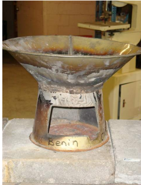
Photo 15: Air intake of Benin benchmark stove.
