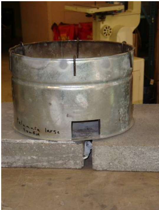
Photo 23: Air intake of Pulumusa.
