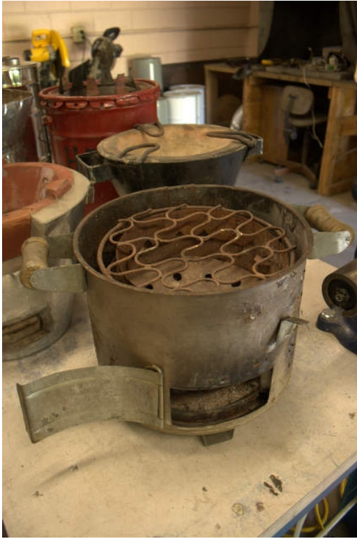
Photo 17: High pot support of Mali stove with door.
