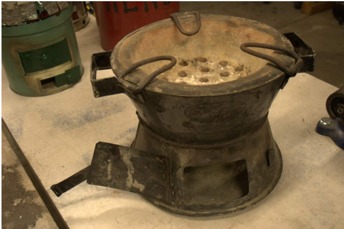
Photo 4: High pot supports of the Jiko with open door.
