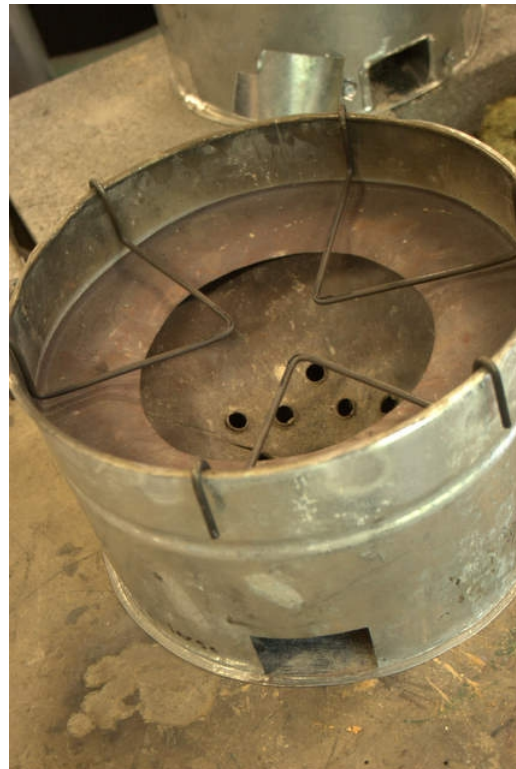
Photo 22: Pot riser of Pulumusa with secondary air and conical fuel bed.
