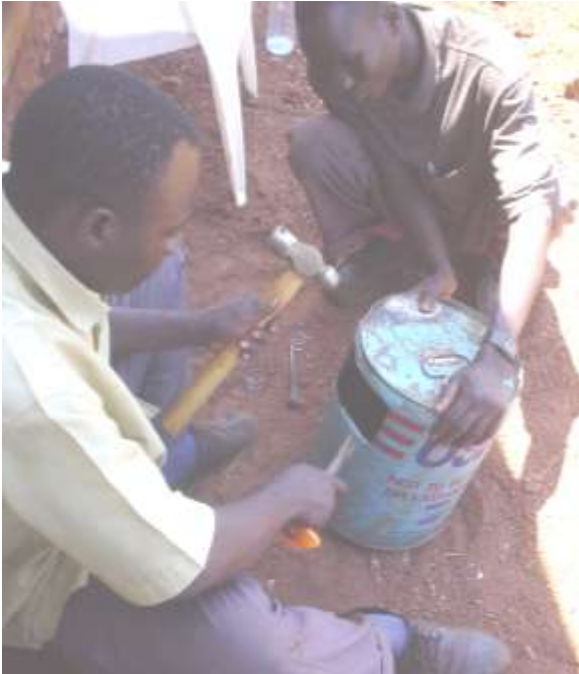
20 liter WFP can being made into a combustion chamber
