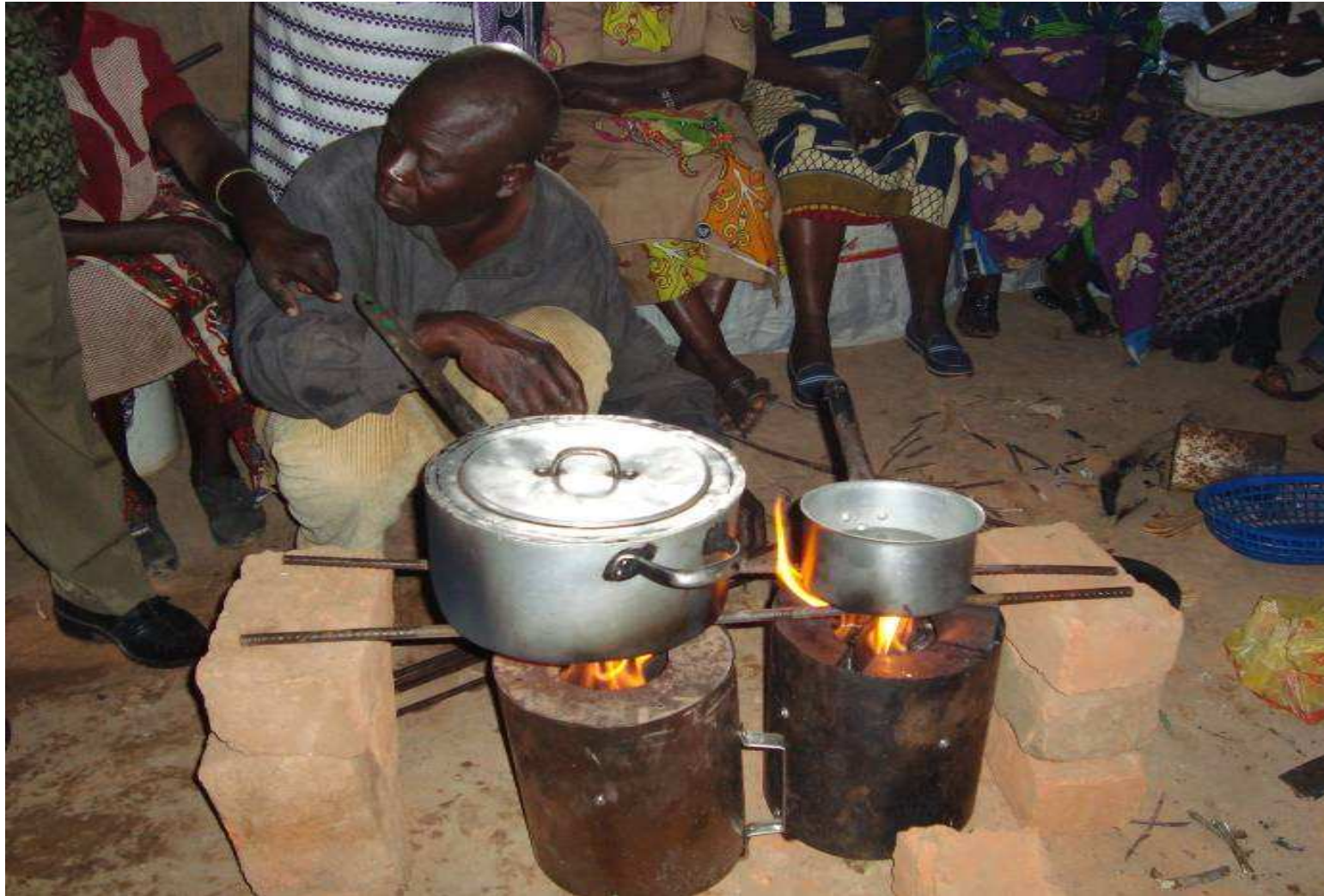
Improved cooking stand to show the flexibility of the TLUD / ND system.
