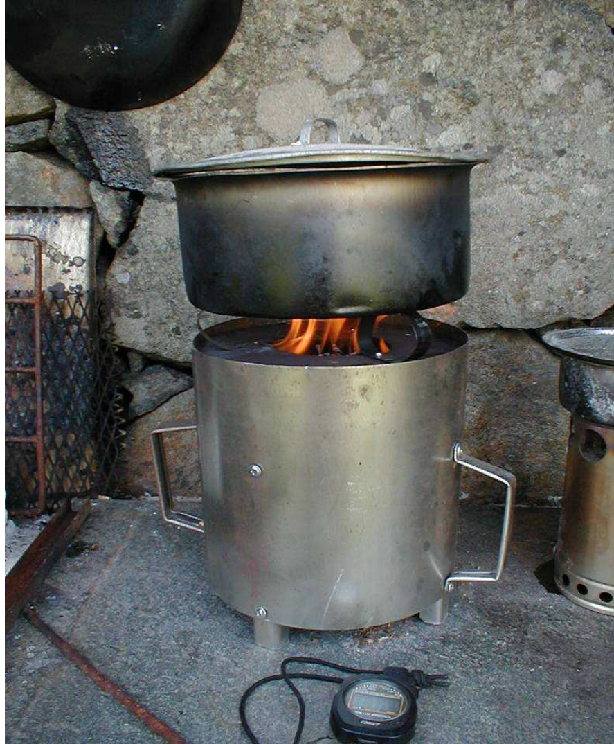
The Peko Pe operating in the burning phase. A minimum of energy is lost to the environment.
