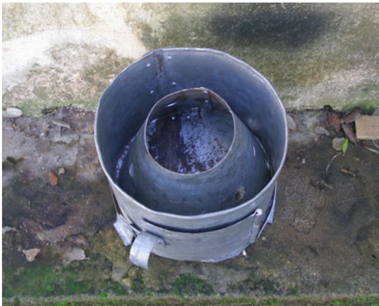
Fig. 5 The cone-shaped cookstove (combustion chamber) with an outer envelope
