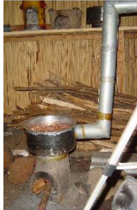
Clay Rocket w/ "pot skirt" & chimney (Rwanda)
