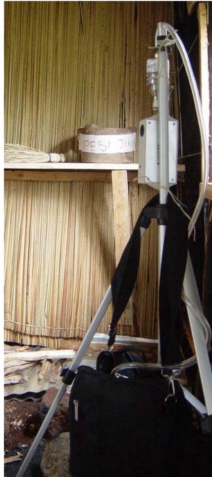
Emissions (CO and PM 2.5 ) monitoring at consistent distance from center of pot
