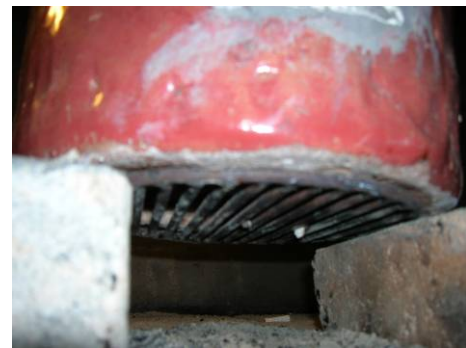
Grate under chimney to hold charcoal
