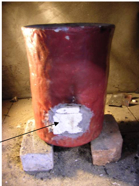
Grate under chimney to hold charcoal
