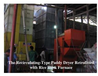
Mr. Clemente P. Abordo, the owner and manager of the Abordo-Portaje Rice Mill in Janiuay, Iloilo has successfully retrofitted his 6-ton capacity Maruyama recirculating-type dryer to a furnace that uses rice husk as fuel. By using the furnace, the cost of fuel and electricity for drying was heavily reduced to P30.00 from P206.00 per hour when using diesel. For 6-ton drying load, Mr Abordo saves as much as P2,464.00 for 14 hours operation .
