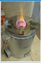
The stove comes into varying models and sizes to suit the availability of fuel in the locality. Biomass fuel like wood charcoal, carbonized coal, or pellets can be used in the stove.
