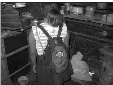
Figure 4 Personal exposure monitoring setup with filter unit in breathing zone and monitor pump inside backpack
