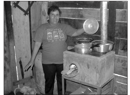
Figure 2 Ecostove with completely enclosed cooking surface (photo: Rogerio de Miranda)
