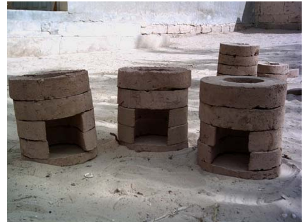
Insulative bricks for rocket combustion chamber
