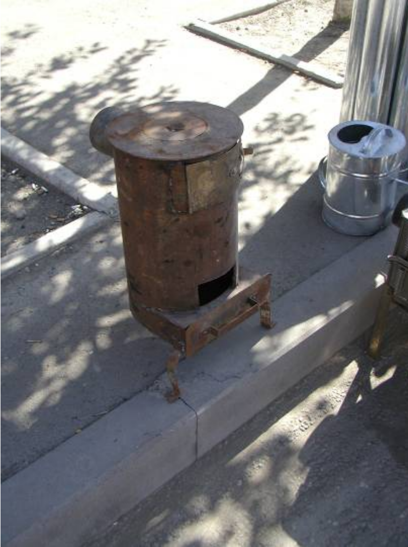
This stove also costs about $15. It has been made from recycled scrap metal. The heavy metal top has a ring to remove so you can heat a pot directly.
