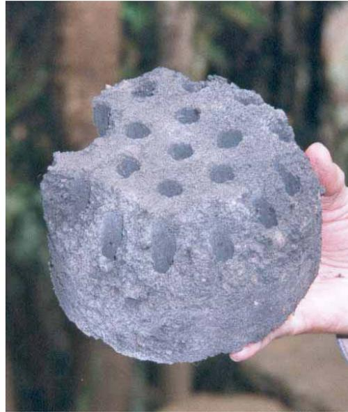
Poor quality briquettes disintegrate during transport
