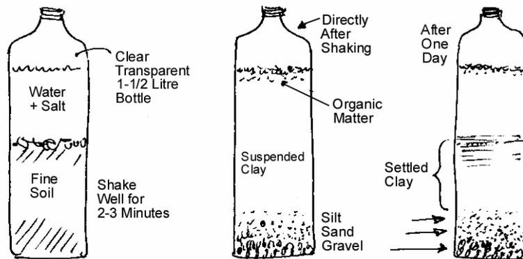
The above test will assist the manufacturer of the briquettes to select the best clay soils. If the soils contain too much sand and silt, these must be washed, using the same principle as with the bottle test. In large tanks the fine clay can be separated in this way. In mixing the dry charcoal material with the fine wet clay, the clay content should be kept as small as possible.
