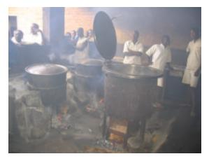
In March 2003, we took the broken stove apart, salvaged most of the material, and rebuilt it as a wood fired rocket stove. Some new sheet metal was used for the combustion chamber but the new Rocket stove could be made, with time permitting, entirely from the used stove. At this point it has not been established if it is more viable for the prisons to retrofit the metal electric stoves or if they should just reuse the stainless steel cooking pot and build a new stove with brick.
