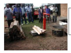
A visual comparison between the quantities of wood used (170kg) for the open fire vs. the amount of wood used (13kg) by the 100L Rocket stove. Independently tested by EP Lauderdale Tea Estates (Malawi).
