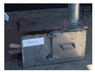
This 2-pot +oven flattop stop was designed for Eastern Produce to replace the expensive and wasteful cast iron Dover stove. The new stove is currently being tested in an Eastern Produce manager's house in Mulanje.
