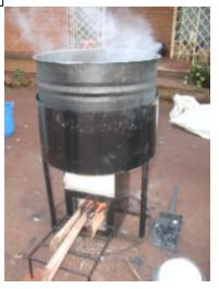
two stoves were made with a slightly skirt and combustion chamber. This was reduce costs and conserve sheet metal enabling us to make two stoves from of 1.6 mm mild steel. The lower skirt will, extent, lower stove efficiency. No testing been done between the two stoves to the difference in efficiency
