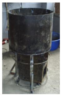
Savepla originally produced this stove as part of the three stoves purchased by ADPP. Unfortunately the stove diameter was too small to fit ADPP's pots. The stove sat unused for three months until I came back. The stove was picked up on Aug 20<sup>th</sup>. and retrofitted with ceramic bricks.. This stove is designed for the taller aluminum 80 L pots that ADPP and WFP both use.
