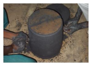
The bucket is turned upside and removed, leaving the stove inverted. A wire is used to cut the stove in half. The stove is dried for three weeks and then fired at 950C for two days. See above brick recipes for possible clay sawdust recipes.
