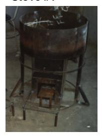
This stove is for Formigas del Futuro. It was built with lower grade clay/sawdust bricks. The liner bricks (with the exception of the two entrance bricks - 'E' on the left and 'C' on the right) were made with common brick clay last year. Although I am skeptical about the durability of these bricks, I thought it would be helpful to make one test stove using these lower quality bricks. If these bricks are successful, than it will greatly simplify production.
