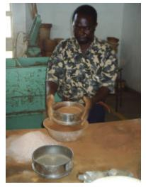
Working with Jameson Mujaye at the National Institute of Scientific Research (NISIR Ceramic Division) we made 5 test bricks, using different mixtures of local high magnesium red clay, mullite grog, and sawdust.
