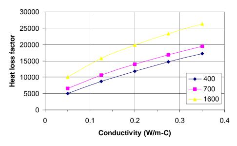
Fig. 1: Heat loss factor vs. thermal conductivity for 30 minutes cooking time with density as a parameter. Density units are kg/m<sup>3</sup>.
