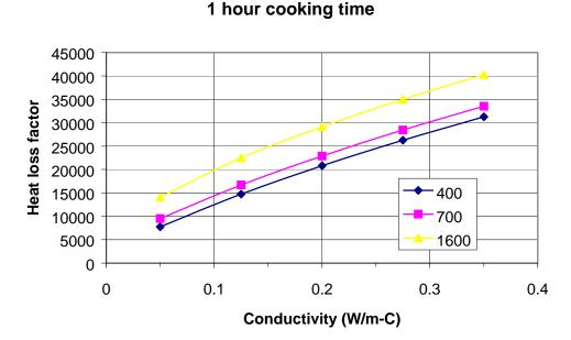
Fig. 3: Heat loss factor vs. thermal conductivity for 60 minutes cooking time with density as a parameter. Density units are kg/m<sup>3</sup>.
