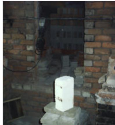
Their current boiler bricks (see photo right) are .9 g/cc, which is heavier than our ideal .6-.7 g/cc brick. However we wanted to compare the durability of their heavier bricks so we worked with them to produce forty .9 g/cc 'heavier' bricks and seventy-two 'lighter' .67 g/cc bricks. These bricks were made with custom moulds that were produced in Mozambique. Measurements in cm
