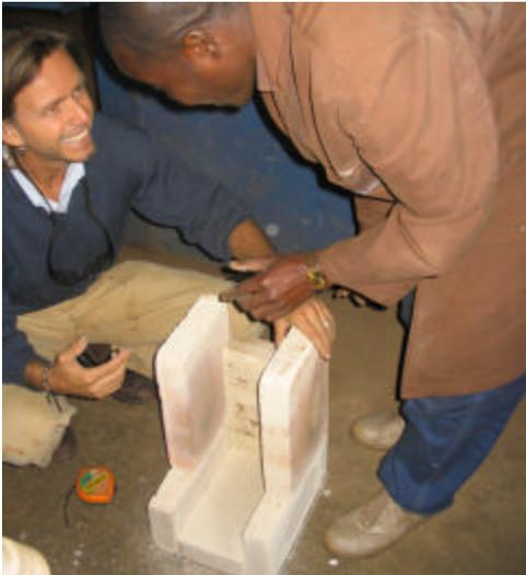
These bricks were then delivered in mid-July and were installed in the 2 mud stoves, the 2 modified WFP stoves, the 2 pot restaurant stove and the Satemwa Tea Estate 110L. The remaining bricks were used to fulfill the first WFP order for 55 stoves. The bricks form the 'L' shaped rocket combustion chamber (see photo left for partially built combustion chamber).
