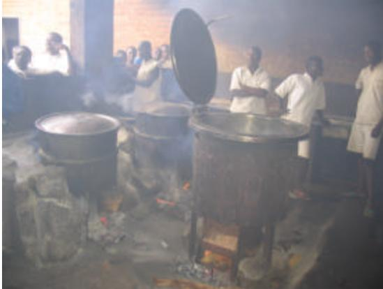
In March 2003, we took the broken stove apart, salvaged most of the material, and rebuilt it as a wood fired rocket stove. Some new sheet metal was used for the combustion chamber but the new Rocket stove could be made, with time permitting, entirely from the used stove. At this point it has not been established if it is more viable for the prisons to retrofit the metal electric stoves or if they should just reuse the stainless steel cooking pot and build a new stove with brick.
